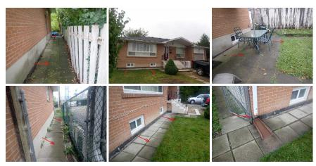
Acceptable, Marginal Vegetation: Trees, Plants - -- Tree limbs over hang the roof and should be cut back to reduce excelled deterioration over the years.
